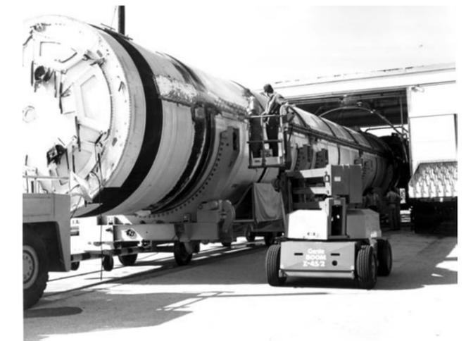
After retrieval post-launch, an SRB is processed through the washing station at Hangar AF.
